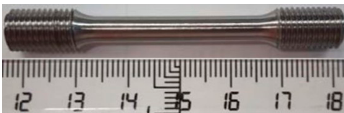
Figure 13. Sample for the mechanical tests of the Ti6Al4V alloy L-PBF used to manufacture our subperiosteal implants.
